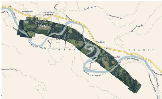
**Figure 3: Our 0.15 m/pixel composite aerial imagery, showing a portion of the Skagit River Valley near Concrete, WA, overlaid on a map of the area.**
