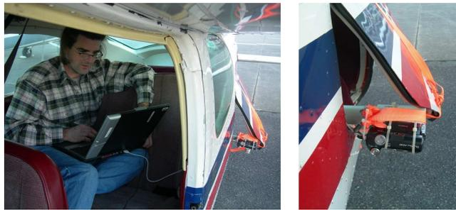
**Figure 2: Our operation: a consumer camera zip-tied to a PVC pipe protruding from a hand-flown Cessna 177.**
